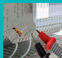
Measure signals during operation, without disconnecting the current loops.
