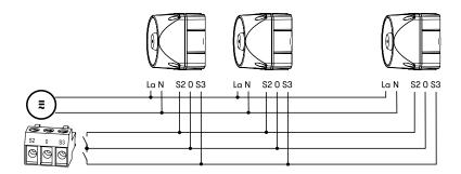
NEW, DIRECT SWITCHING VIA 4 TERMINAL POINTS WITH A COMMON CONNECTION POINT, N
