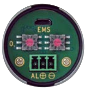
Thermalert 4.0 supports 2-wire loop
