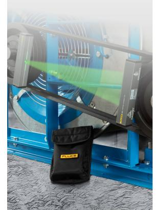
It is a known fact that all rotating machinery are susceptible to misalignment. An aligned pulley system reduces belt wear, power losses, and vibration of machinery, leading to improved performance.
