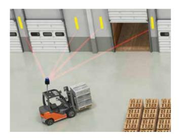
LGS-N50 is suitable for navigation of AGVs moving up to 2 m/s, has a scan rate selectable up to 25 Hz and 60.000 measurements per second.
