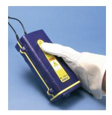
Press and hold operate button. Open mold after 10 seconds.
